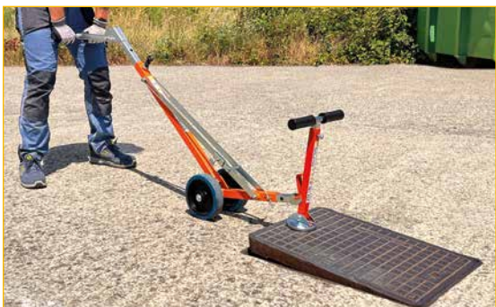
Lifting with wheeled levers APS80 or APS90
