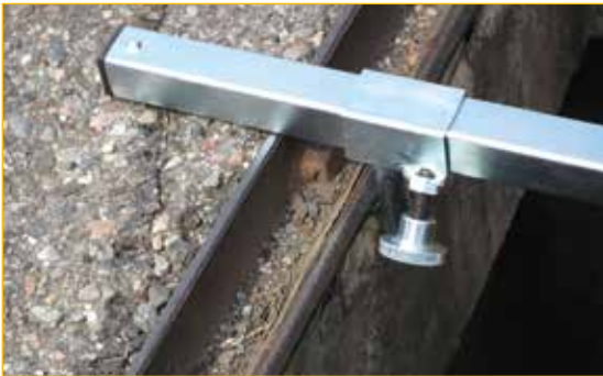
Sliding and adjustable struts at the tip of the arms to keep the cross in the correct position.
